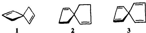
Fig 1. R or 4S - spiro[3.3]hepta - 1,5 - diene (1), R or 5S - spiro[4.4]nona - 1,6 - diene (2) according to the old and new method of the Cahn, Ingold, Prelog convention, 8 respectively, and spiro[4.4]nonatetraene (3).
